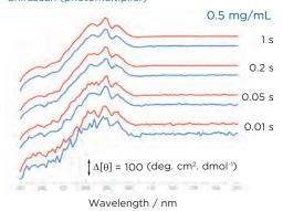
Tertiary structure of lysozyme – raw data, no smoothing, baseline corrected, n=3 scans, 1 nm step, 10 mm pathlength, spectra offset for clarity
