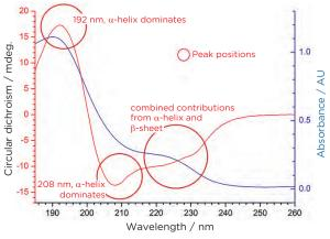
Simultaneous acquisition of CD and absorbance spectra, 0.5 mm pathlength, Chirascan V100. Courtesy of leading research university, Germany
