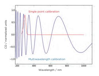
Conventional chemical calibration methods require considerable skill in preparation. Standards, such as camphor-10-sulfonic acid (CSA), are unstable, photolabile and hygroscopic. In addition, single wavelength calibration (290.5 nm) assumes the same linear response at all wavelengths.
