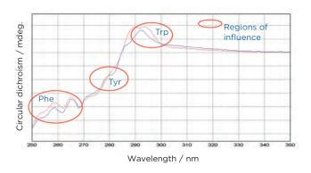
Differences between near-UV spectra due to slight changes in orientation of aromatic moieties, Chirascan V100, 10 mm pathlength
