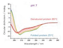
Two of six denaturation datasets acquired at pH 2-7, lysozyme, Chirascan 6-cell turret, Chirascan V100, raw data, no baseline adjustment, no smoothing, 0.5 mm pathlength
