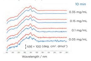
Tertiary structure of lysozyme – raw data, no smoothing, 10 min. baseline / 10 min. sampling, n=3 scans, 0.5 nm step, 10 mm pathlength, spectra offset for clarity
