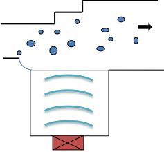
Matec's patent-pending acoustic sensor provides acoustic attenuation spectroscopy measurements without sample dilution and without the use of moving parts.
